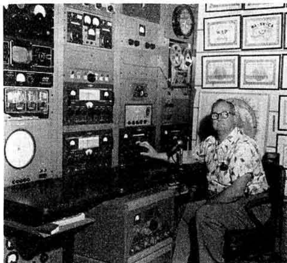
W6YY of La Canada, California, is one of the best known calls in the world. The equipment includes separate exciters, 4-1000A power amplifiers and aerials for each of the h.f. bands, with a common modulator and power supplies. Vertical aerials are used on 1-8 Mc/s and 3-5 Mc/s with beams for the other bands. The two receivers are a Collins 75A2 and a 75A4.
